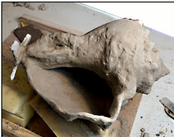
PLASTER MOLD FOR SLIP CASTING
