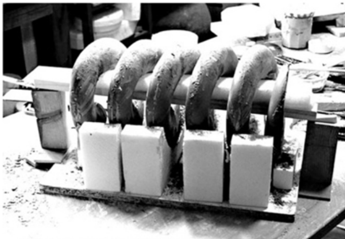
ASSEMBLY OF 12 CLAY SLIP CASTINGS CREATED FROM THE PLASTER MOLD OF THE MODULE
