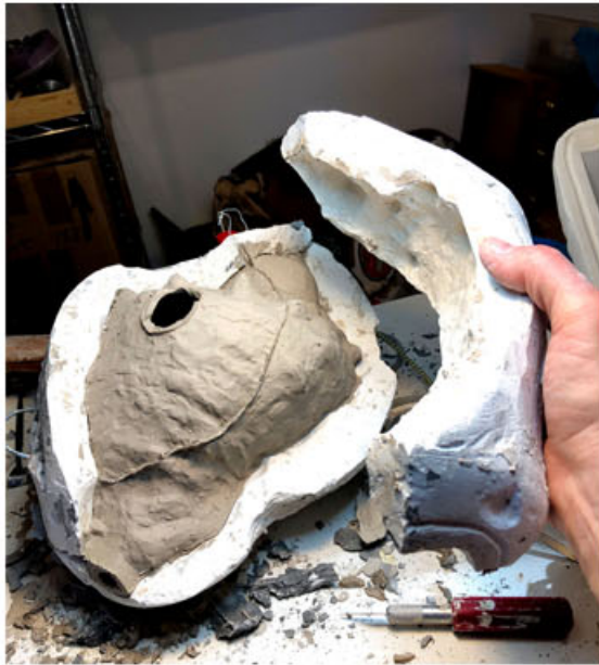
PLASTER MOLD FOR SLIP CASTING
